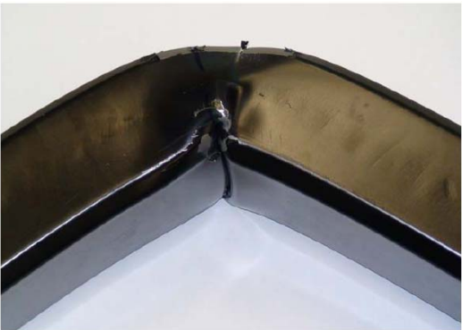
foam filled beam 21,15 kg
