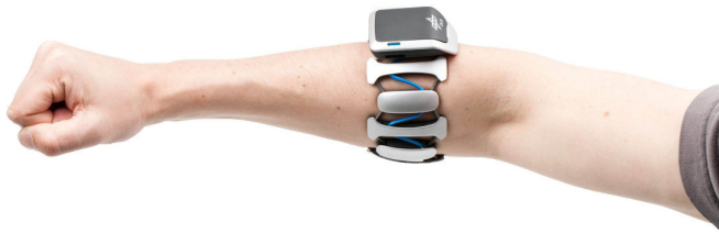
Fig. 10: VibroTac in stretched state with correct positioned segments
