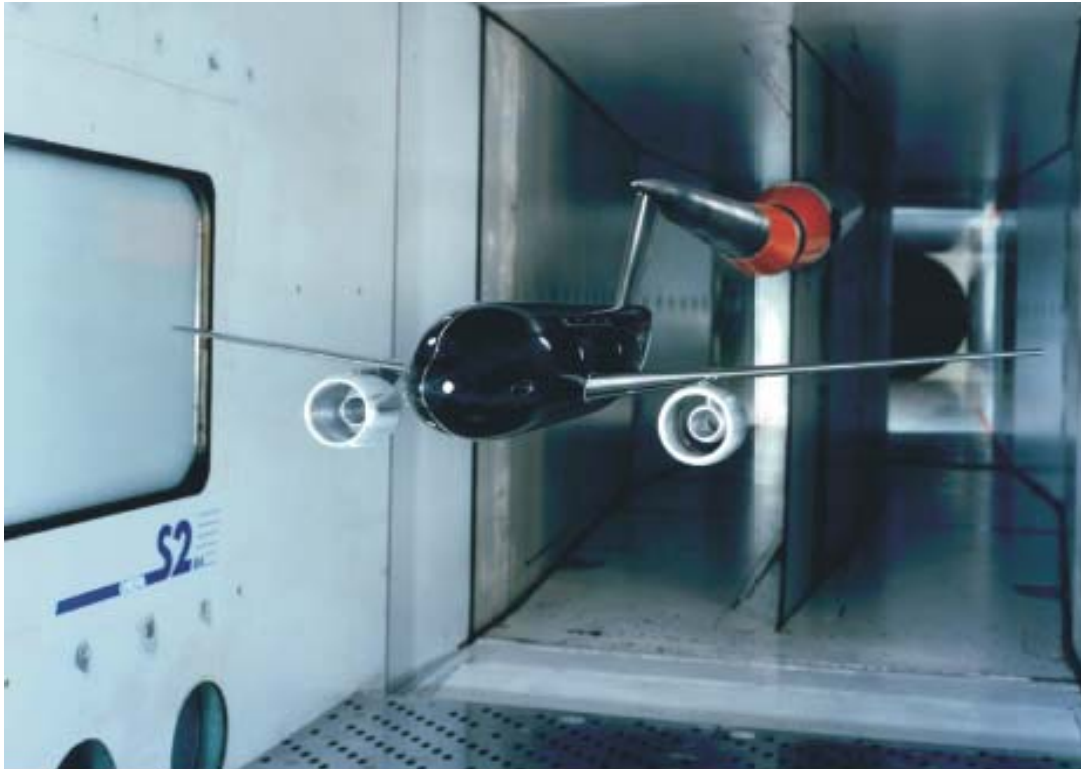
Fig. 1 DLR-F6 with VHBR nacelles in ONERA S2MA wind tunnel.
