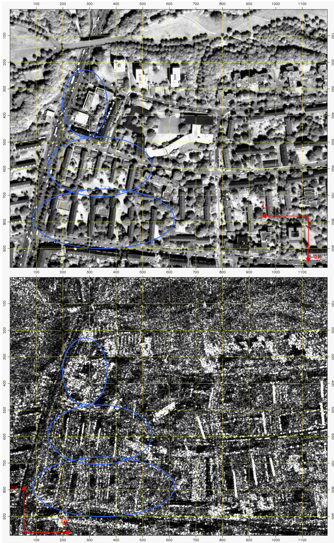
Figure 6. Part of Munich city acquired by IKONOS (upper image) and TS-X (lower image) using the accidental satellite formation. Yellow grid lines are for better orientation between two images. Red arrows show flight (az) and look (rg) directions.
