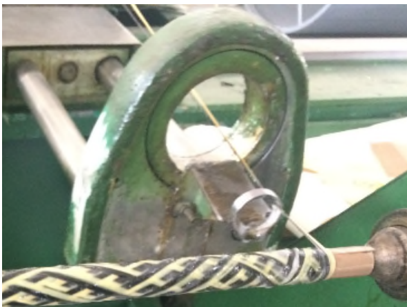
Figure 6: Winding of helix layer
