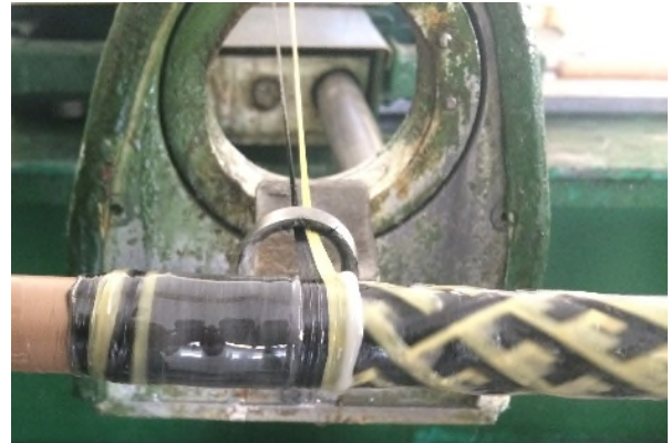
Figure 7: Winding of hoop layer
