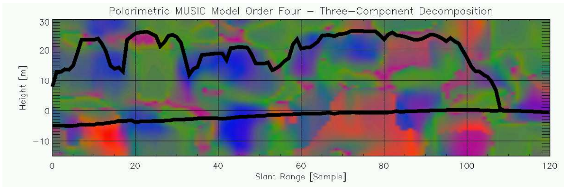
Figure 2: Three-component decomposition of polarimetric MUSIC with model order four: Double-bounce red, surface reflection blue, volume diffusion green.
