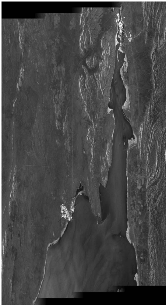
Fig. 5. TOPSAR acquisition in February 2009 in South Australia; the scene extension in range (horizontal) is about 100 km. The scene dimension and resolution (16 m) is as in TerraSAR-X ScanSAR products.
