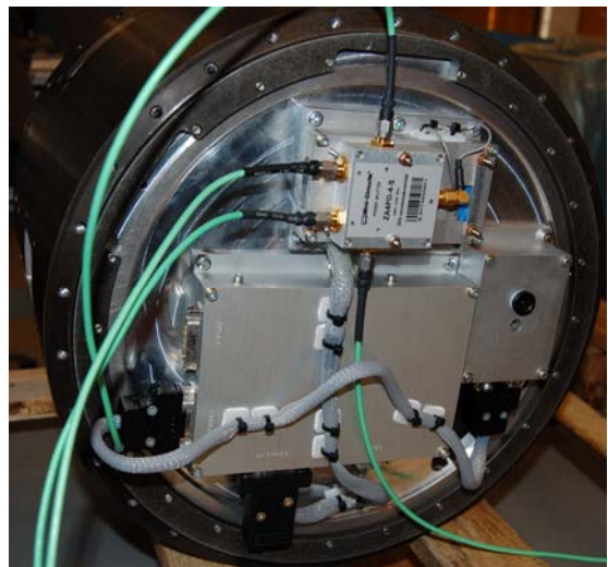
Figure 7. HISPICO system mounted on bulkhead (from top left to bottom right): HISPICO with power splitter, power control and data handling unit (PCDH), camera
