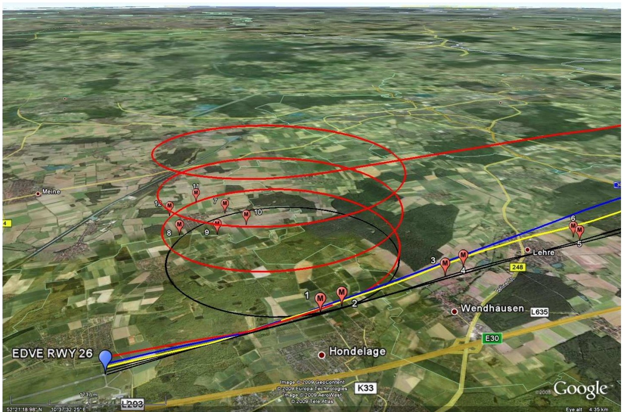
Figure 7. Flight ground tracks (black), flight paths (yellow: reference, blue: steep, red: HeNAP), and observer locations around EDVE (Google Earth)
