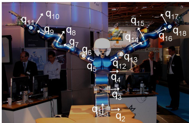
Fig. 1. The table-mounted Justin . The joints q_{1..18} relevant to the described inverse kinematics algorithm are shown.
