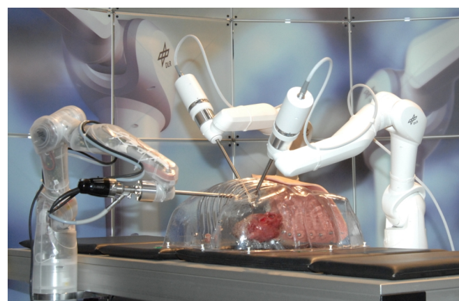
Fig. 1. The remote telemanipulator of the DLR system for minimal invasive robotic surgery, three versatile light-weight robots MIRO with 7 DoF and torque control, two surgical instruments with force-torque sensing, one stereo endoscope.
