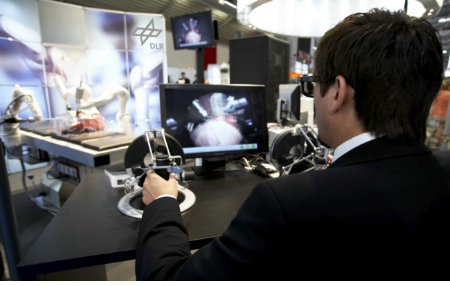
Fig. 2. The teleoperator station for the surgeon, two haptic master devices and a stereo display.
