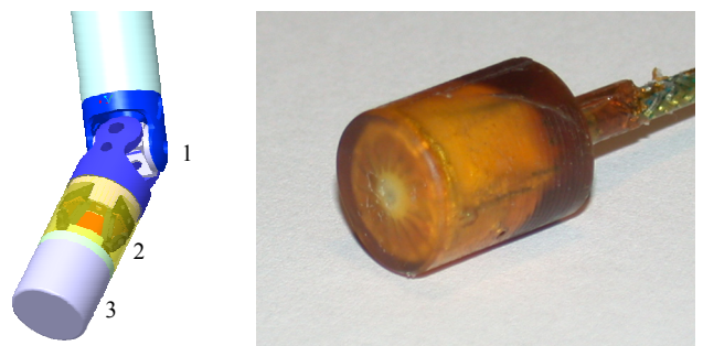
Fig. 1 Left: Planned integration in the existing DLR MIRS instruments; 1) universal joint, 2) 6 DoF force/torque sensor, 3) ultrasonic probe. Right: First Prototype of the unidirectional ultrasonic probe ( \varnothing 10\text{mm} ).
