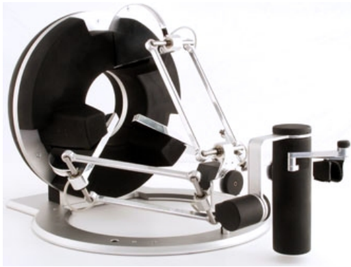
Fig. 4 Haptic interface “omega.7” by ForceDimension, Inc., Lausanne, Switzerland. The system provides 3 passive (rotational) and 4 active (translational and functional) DoF. Photo: ForceDimension [15].
