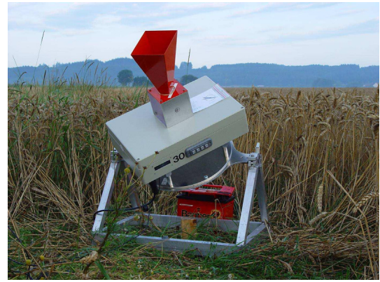
Fig. 3. DLR ground receiver deployed for receiving radar pulses.
