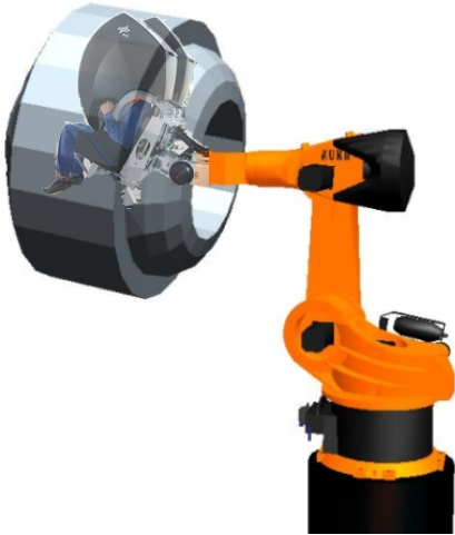
Figure 5. Enveloping rotationally-symmetrical volume, mounted to the robot's tool flange
