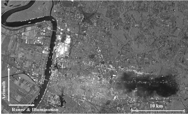
Fig. 6: An example of a SAR image with rain-cell signatures recorded with TerraSAR-X in the US close to Baton Rouge. The white shading to the left of the dark spot is due to direct reflections from the rain region. The darkly shaded areas are due to rain attenuated (blocked) signals from the ground.
