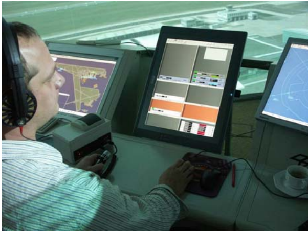
Figure 4: A-SMGCS Ground Equipment: EFS plus CPDLC functions integrated at the Controller Working Position of ATS
