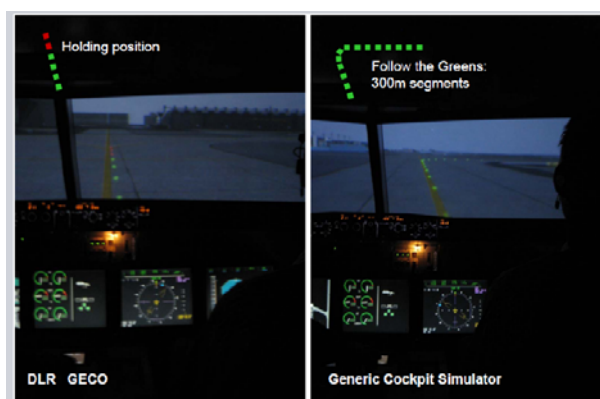
Figure 10: GECO cockpit view while being guided by individually switched taxi light segments [19][Picture provided by Siemens]
