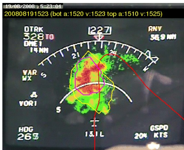
Figure 13: On board radar screen and Wims Cb objects for 15h23 on 19 august. Magenta and yellow contours show bottom objects of severity level 2 and 1 and are 3 minutes forecast. Red line is the aircraft actual track.
