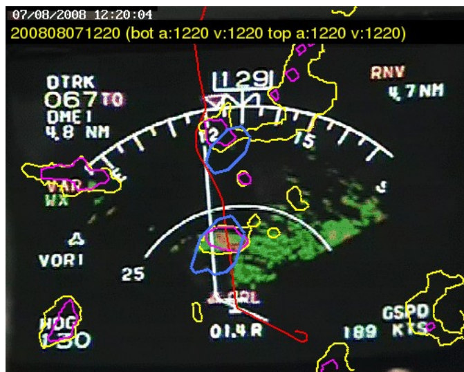
Figure 16: On board radar image for 7 August, 12h20 UTC. Contours as in previous figures, except for the addition of blue contours showing the satellite depiction of developing cells
