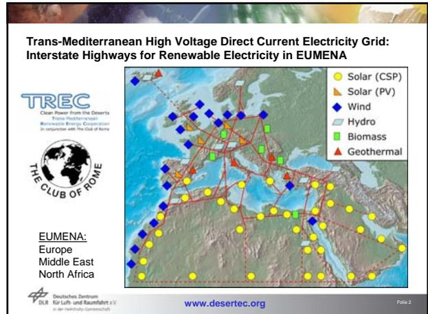
**Trans-Mediterranean High Voltage Direct Current Electricity Grid: Interstate Highways for Renewable Electricity in EUMENA**
