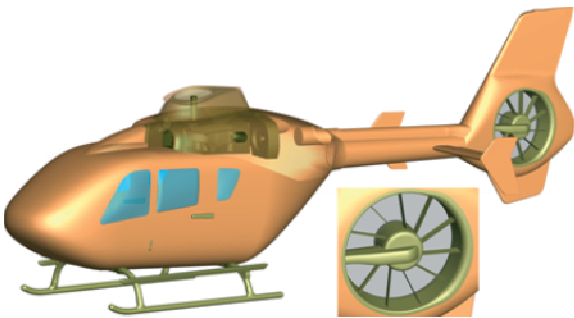
Figure 14: CATIA model of the EC135 isolated fuselage including Fenestron® and engine deck
