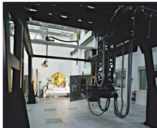
Fig. 21: European Proximity Operations Simulator – EPOS (DLR, German Space Operations Center) Utilized for Long-Range Docking Maneuvers Within CX-OLEV
