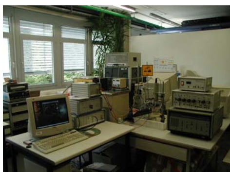
Fig.1: Experimental set-up for the electrochemical characterisation of Ni-electrodes in alkaline solution
