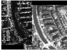
Figure 1. GIS overlay of a TerraSAR-X and an Ikonos image
