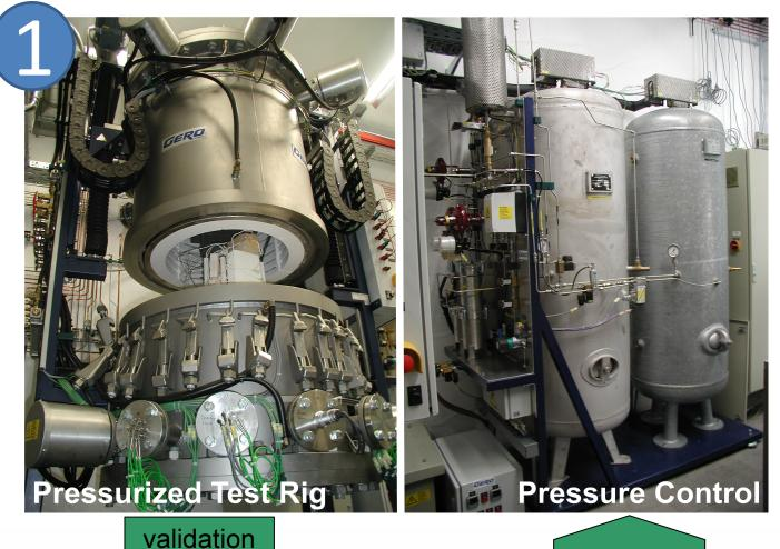
**Pressurized SOFC systems for** stationary applications
