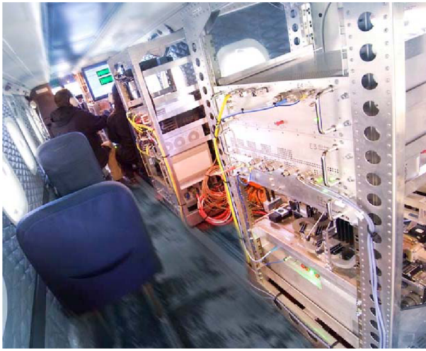
Fig. 5. F-SAR system installed onboard DO228 aircraft for flight testing in X-band.
