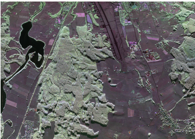
Fig. 10. Quadpol S-band image acquired by F-SAR (5km maximum swath from 3000m flight height)
