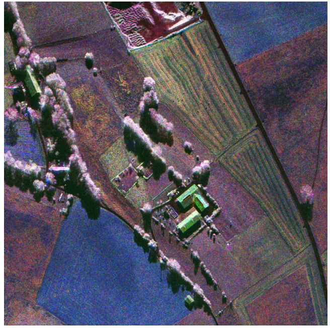
Fig. 7. Zoom into a F-SAR quadpol X-band image. Spatial resolution 0.4m
