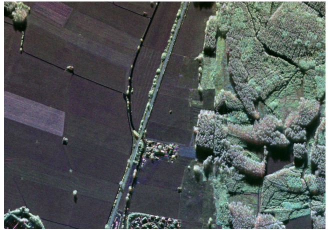
Fig. 11. Zoom into a F-SAR quadpol S-band image of Fig. 10. Spatial resolution 0.5m
