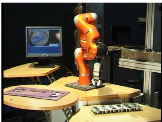
Figure 5: A light-weight robot arm as an assistant for human-like working in industrial environments the PAPAS experimental setup is designed to demonstrate a typical example of an industrial manufacturing process.
