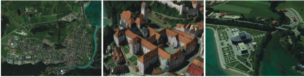
Figure E.1: Visualization of a reconstruction of Fuessen. The images cover an area of 24 km 2 and have a ground resolution of 15 cm/pixel, leading to a DEM and ortho-image consisting of 1 billion height values and pixels.
