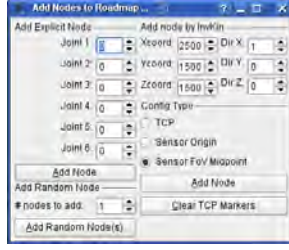
Figure D.4: Tab window for adding nodes. Left: Adding nodes by joint angles. Right: Adding nodes by TCP, F_{sensor} , or FoV to the roadmap.
