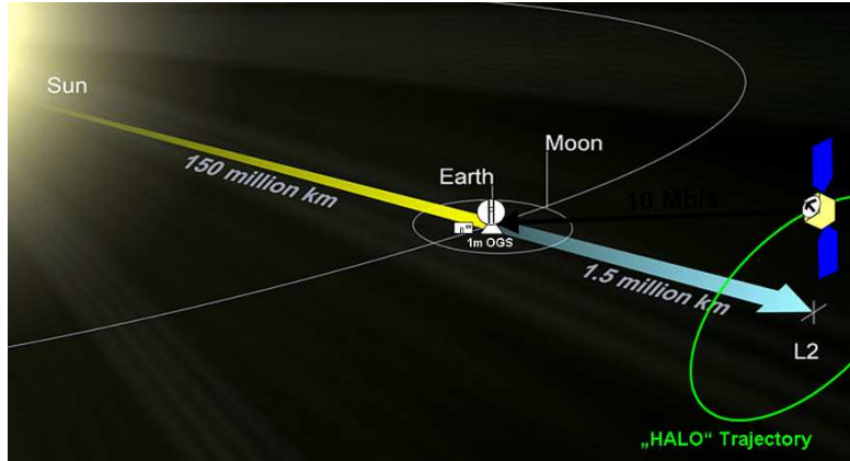
Figure 3: DOLCE mission scenario - optical telemetry link from L2 to OGS on Earth
