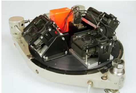
Fig 2 DLR 3K-camera system consisting of three Canon EOS 1Ds Mark II, integrated in a ZEISS aerial camera mount
