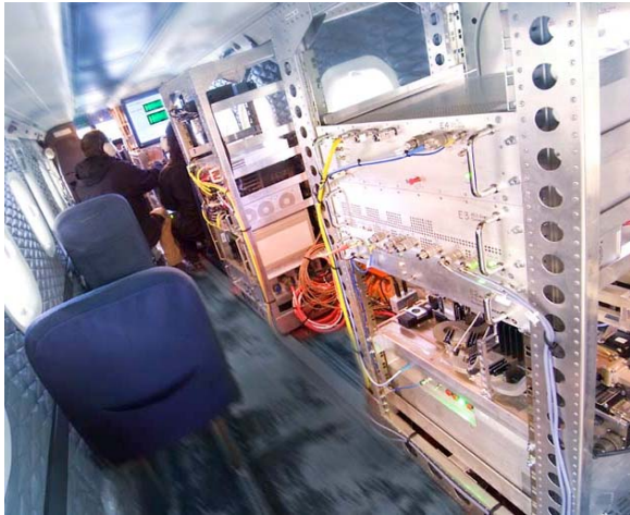
Figure 5 F-SAR system installed onboard DO228 aircraft for flight testing in X-band.
