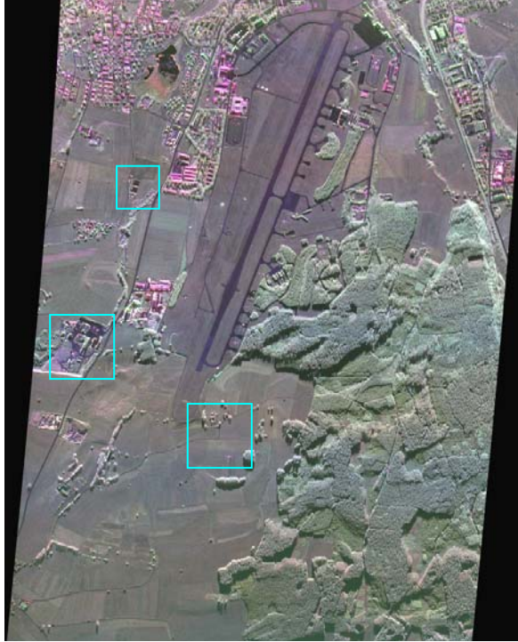
Figure 7 F-SAR image result, X-band polarimetric (HH: red, HV: green, VV: blue), bandwidth 300MHz. Calibration test site Kaufbeuren (Germany). Details marked in light blue.
