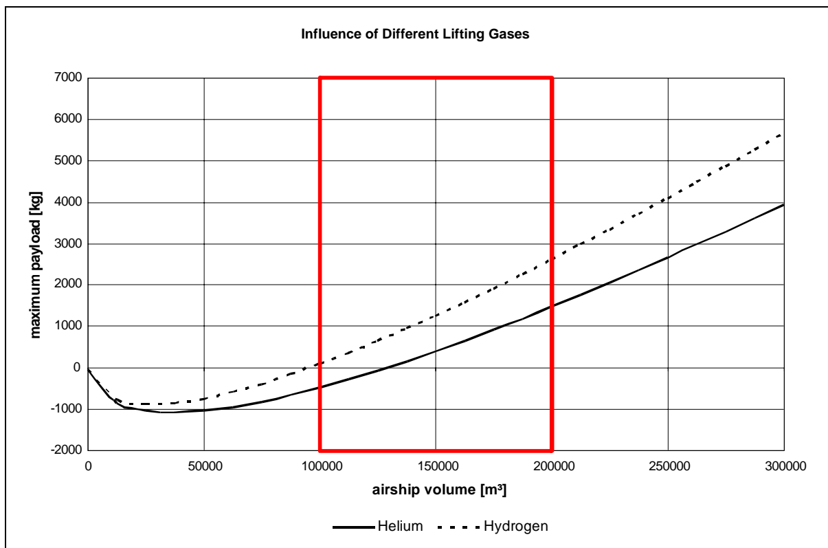
Figure 49 Variation of useful payload with airship volume for two types of lifting gas: helium (solid line) and hydrogen (dashed line).
