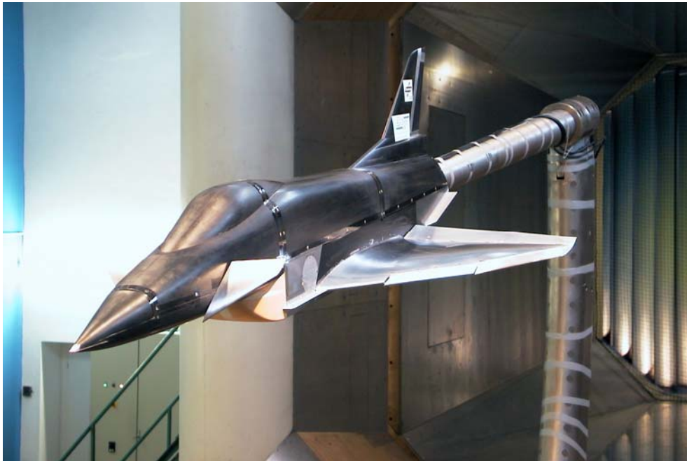
Figure 3: X-31 Remote control model in the DNW-NWB Braunschweig.
