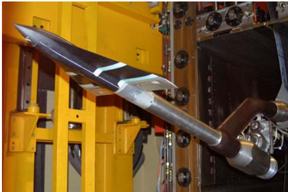
Figure 3: 65°-swept delta-wing-fuselage-model-configuration with remote controlled trailing-edge flaps on the roll-rig device in the DNW-TWG Göttingen.
