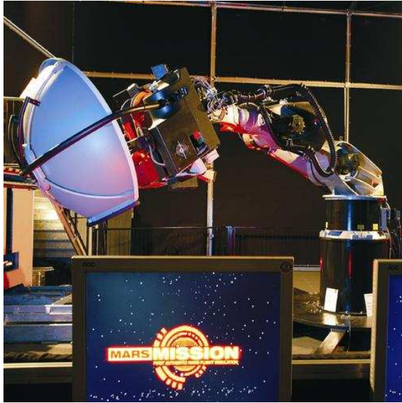
Figure 1: Robocoaster equipped with a spherical projection screen (left) and with two retractable caps, containing LCD screens and sound systems (right), source: DLR
