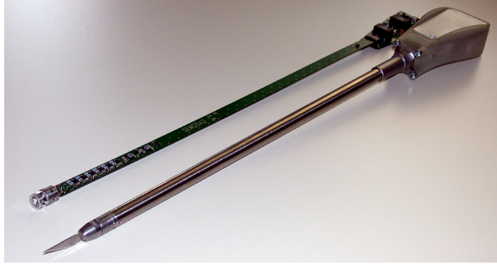
Fig. 4. Sensorized scalpel with force/torque sensor at tip and electronics.
