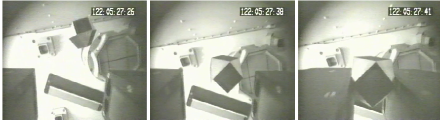
Fig. 4. One of the pioneering experiments in ROTEX has been the fully automatic grasping of a free-flying object from ground despite a varying round-trip-delay of up to 7 seconds.
