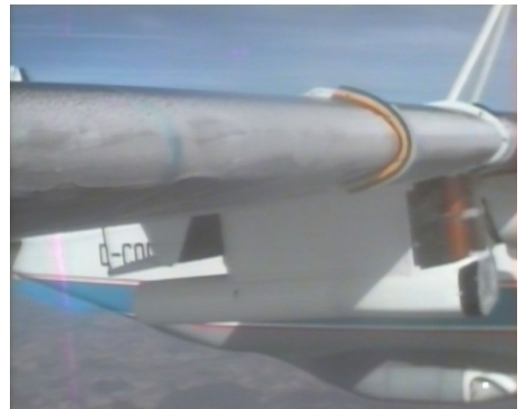
Figure 20. Ice accretion on the Do 228 wing after a few minutes of spraying.
