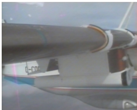
Figure 22. Clean wing before water spraying with discs installed for measuring the ice thickness. View is from the wing tip mounted camera.
