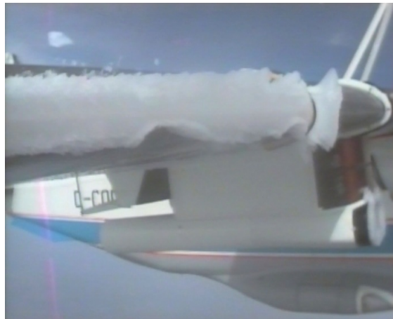
Figure 23. Ice shape on the laminar glove after 13 minutes of water spraying on the Do228 wing short before ice shedding.
