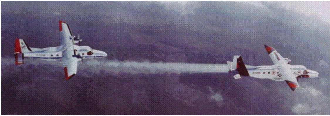
Figure 15. DLR test aircraft Do228 in the water spray plume of the Dornier icing tanker aircraft.
