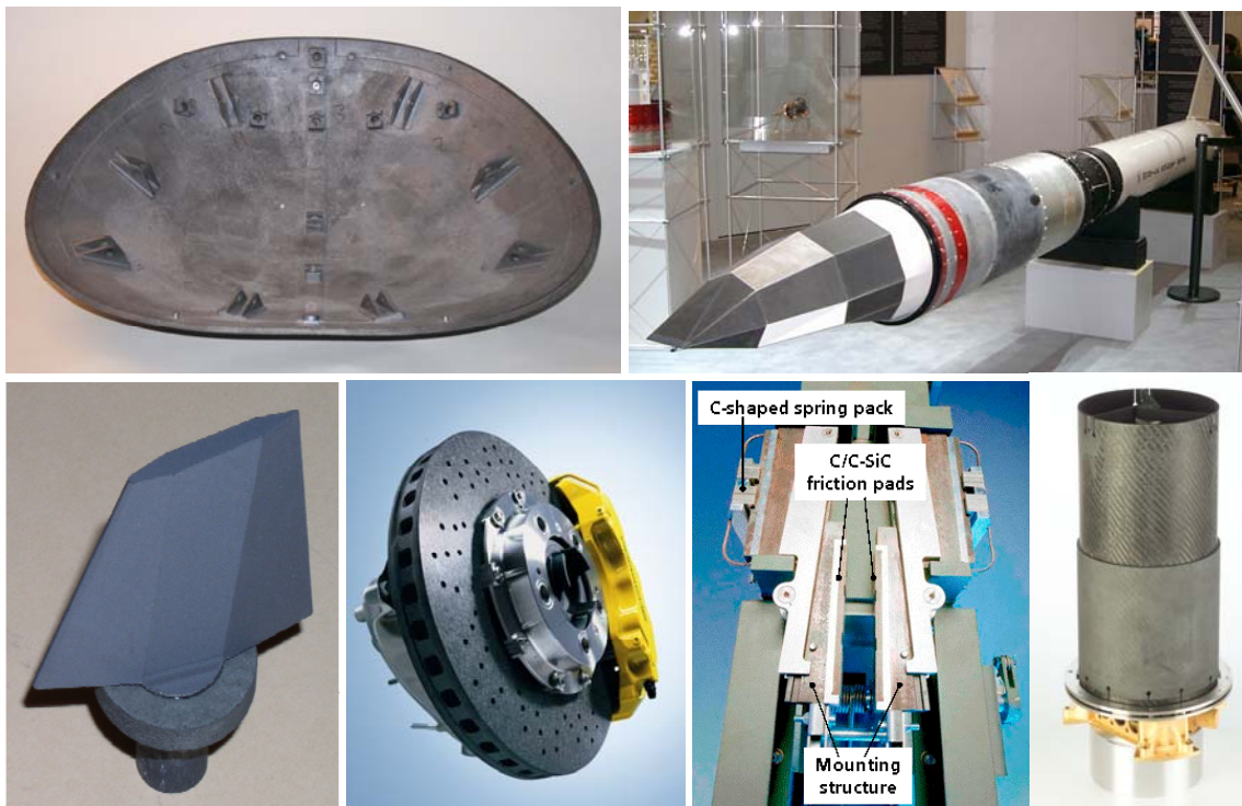
Figure 38. Exemplary C-fibre reinforced SiC parts manufactured via MI / LSI. Top left: Nose cap (ca. 740 x 640 x 170 mm 3 ; t ca. 6 mm; m ca. 7 kg, DLR) for X 38. Rear side showing in situ joint load bearing elements. Top right: Facetted TPS structure, built up by flat panels, mounted on a rocket system. Bottom from left to right: Jet vane (ca. 60 mm x 60 mm) and sealing ring for TVC of missiles (DLR). Porsche Ceramic Brake Disk (PCCB) based on short fibre reinforced C/SiC (Porsche). Elevator emergency brake system with C/C-SiC brake pads 142 mm x 34 mm x 6 mm. In situ joint telescope tube (Ø 140 mm, l = 160 mm, t = 3 mm) for the laser communication terminal in the satellite TerraSAR-X (Zeiss Optroniks / DLR).
