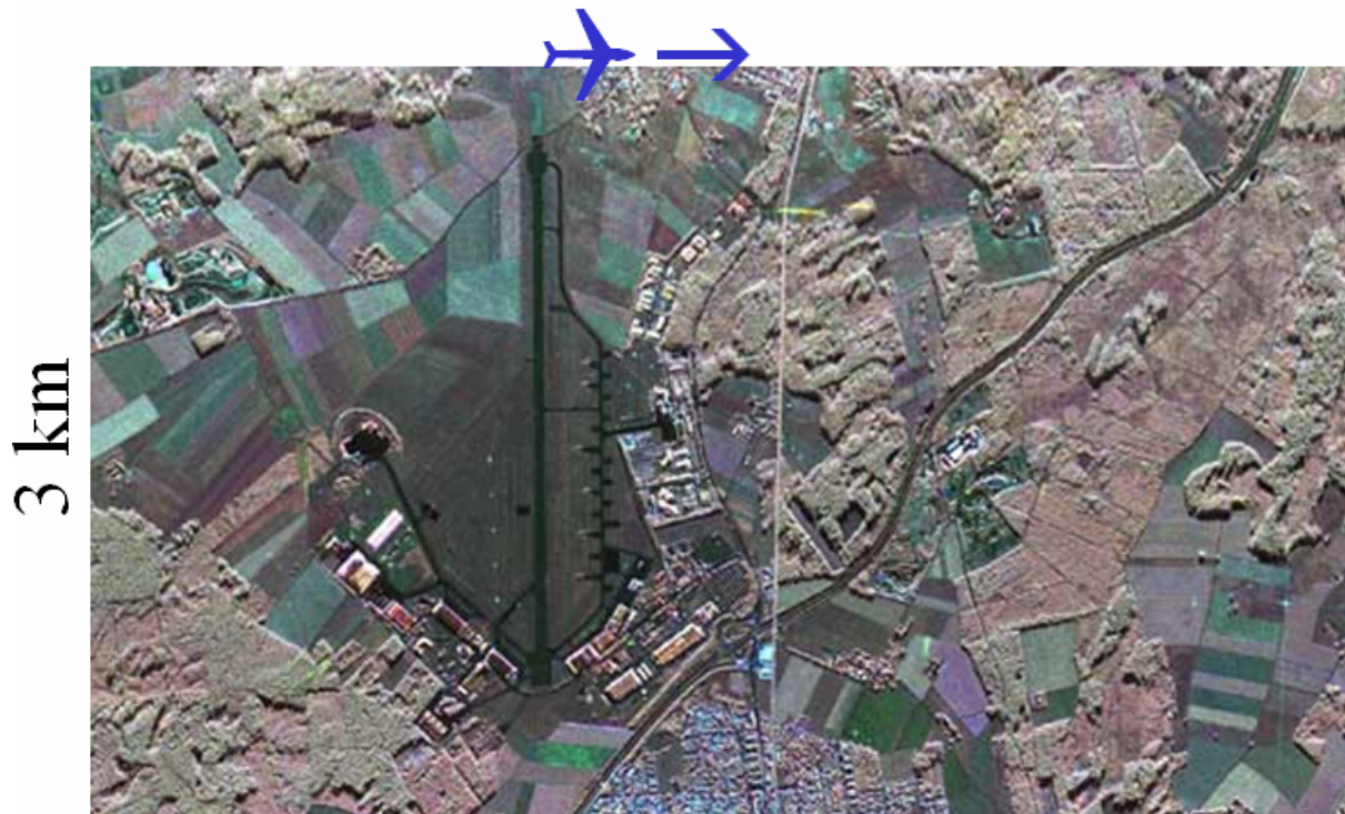
Figure 2. Fully polarimetric SAR image of Oberpfaffenhofen, including DLR facilities in image center. Composite obtained from 2 dual-polarized data takes in C-band (HH-green, HV-red, VV-blue).
