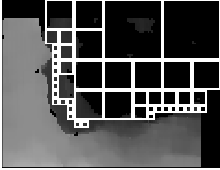
FIG. 10: Depth image example and the dark regions found, marked with squares. Flight Corridors around the center of every region are searched.
