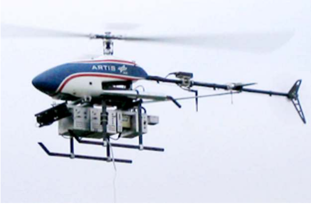
FIG. 2: The helicopter ARTIS with an on-board stereo camera.
