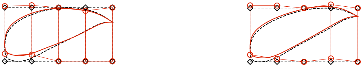
Figure 36. Parametrized lattice box and wing sections IV and V for initial (dashed) and deformed (solid) grid.
