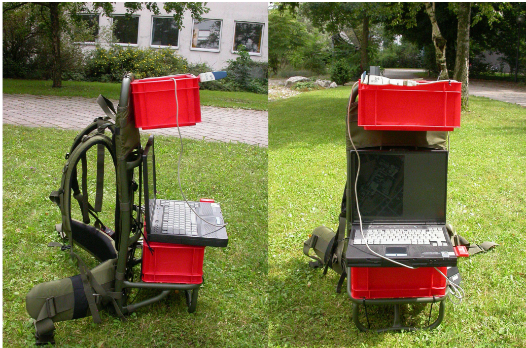
Figure 5.1: The backpack equipped with the laptop, the 3G/GPRS data card, the bluetooth adapter, the bluetooth GPS receiver and the electrical compass.
