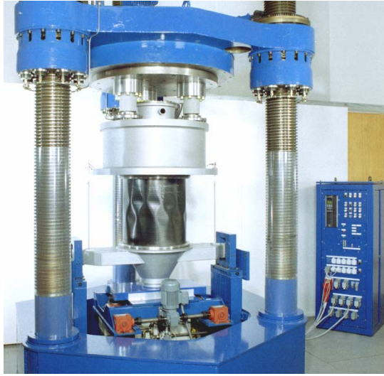
Figure 1. Photo of DLR’s buckling test facility.
