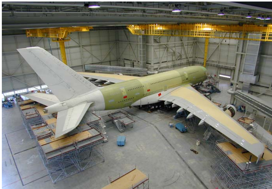
Figure 5 – Ground Vibration Tests on Airbus A380-800 (Copyright Airbus S.A.S.).
