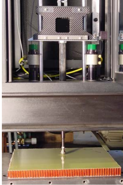
Figure 4: Impact facility at ILR Dresden [14].
