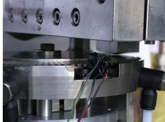
Fig.1 Mounting Position of the pressure modulator device for transversal mode test
