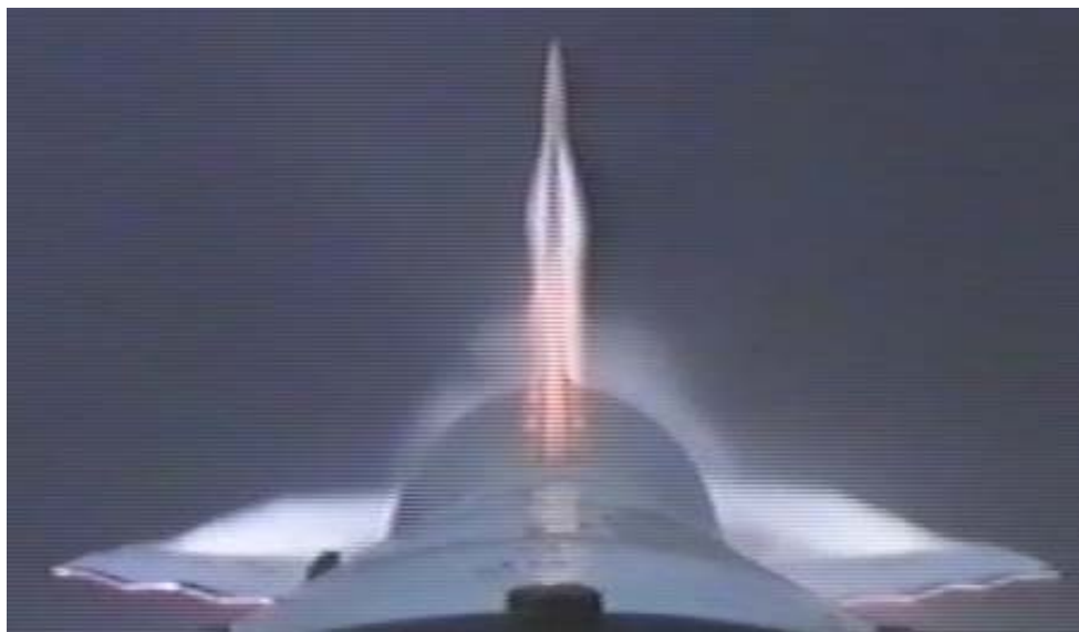
Figure 16. Visible Evidence of Thermal Loads on the 2 nd Stage Fins
