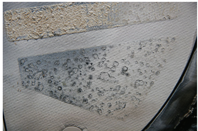
Figure 23: Titanium-dioxide and Yttrium-titanium coating after flight.
