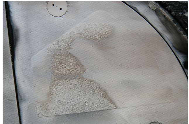
Figure 22: Yttrium-silicate coating after flight.
