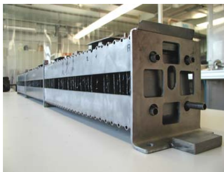
Test modules in the power range of 10 – 100 kW for different of PCM storage design concepts
