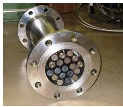
Test modules in the power range of 10 – 100 kW for different of PCM storage design concepts
