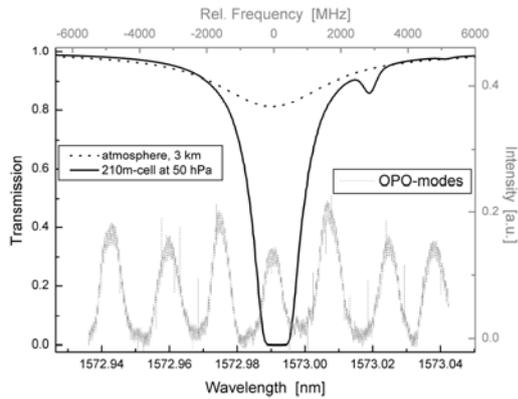
Fig. 3: Calculated transmission of an atmospheric measurement path of 3 km (370 ppm CO<sub>2</sub> concentration) and of the 210-m cell in relation to the OPO resonator modes. The modes have been measured using the seed laser.
