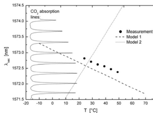
Fig. 2: Measured and calculated temperature tuning curves of the signal wavelength of the NCPM OPO. The obtained wavelengths match favorably to the CO<sub>2</sub> absorption lines. Model 2 (using Sellmeier and thermo-optic coefficients from [6]) fails to precisely predict the wavelengths while model 1 (according to [7]) gives much more realistic results. The tuning range can further be extended by tuning the pump wavelength.
