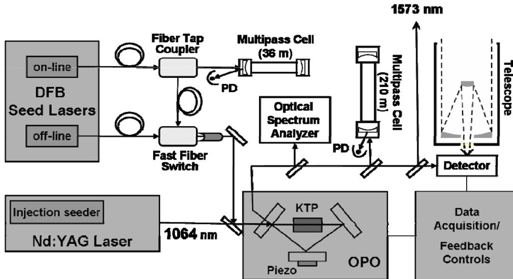
Fig. 1: Schematic set-up of the transceiver system
