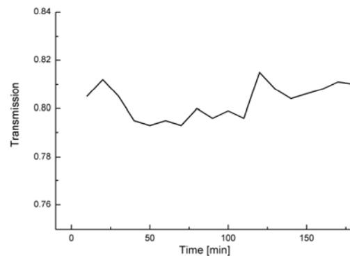
Fig. 4: Measurement (10-minute average) of the atmospheric transmission due to CO<sub>2</sub> absorption. The distance from the lidar to the topographic target was 1.5km (one way). The transmission thus matches well to the calculated value of ~80% (see Fig. 3).
