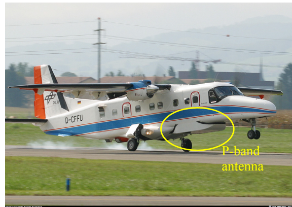
Figure 5 E-SAR onboard DLR's Dornier DO228-212 aircraft touching down after a successful measurement flight.
